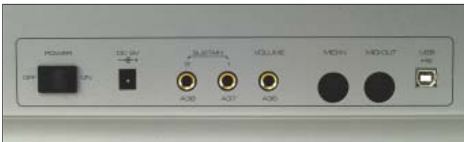
The Pro 88 can be used as a standalone MIDI controller when powered via a 9V adapter. Note that the controller jacks are labeled with their controller block and number for manual-free reference.
